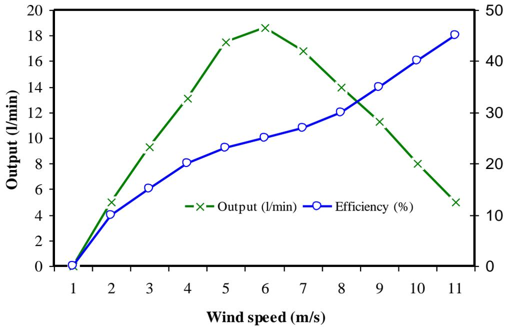
Figure 6. Wind pumps output and efficiency.
