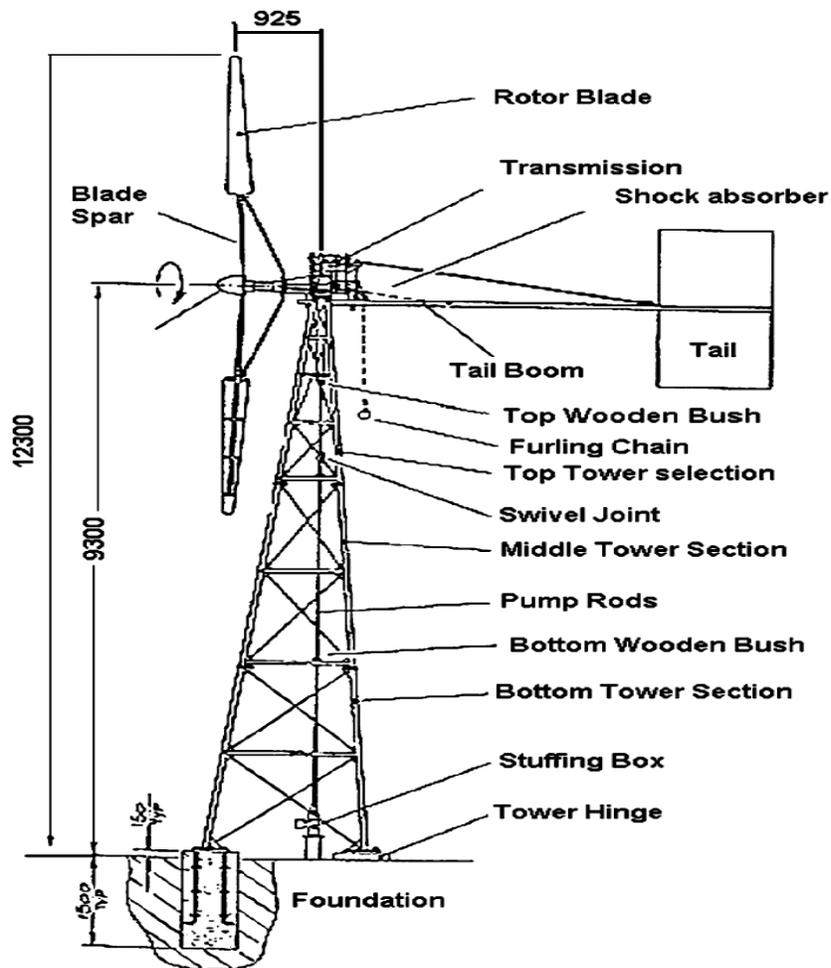
Figure 3. Schematic of the construction of the wind pump.
